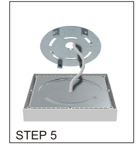
STEP 5 Push and feed all wires up into Junction Box as you raise the fixture up into place
