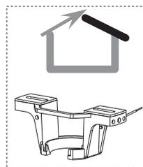
**This fan cannot be used for the ceiling which angle is greater than 19 degree.**
