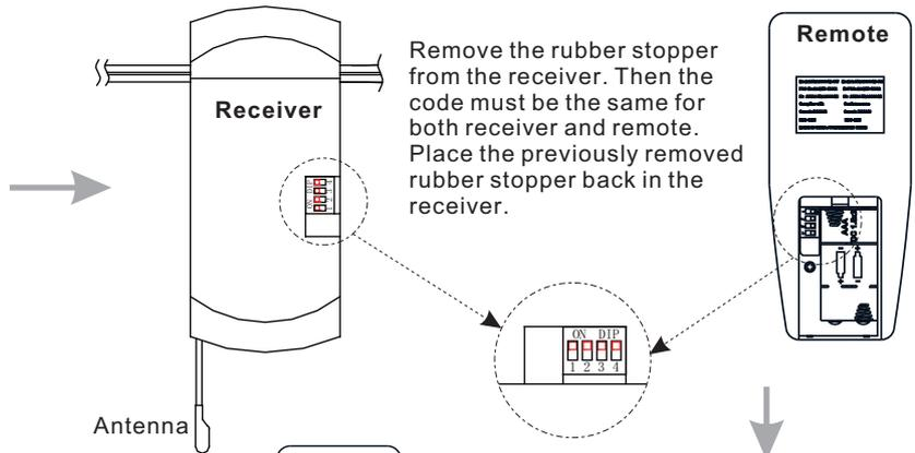
Remove the rubber stopper from the receiver. Then the code must be the same for both receiver and remote. Place the previously removed rubber stopper back in the receiver.
